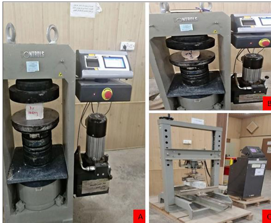
Figure 2. Mechanical tests of geopolymer concrete: (a) compressive strength, (b) splitting tensile strength, (c) flexural strength
