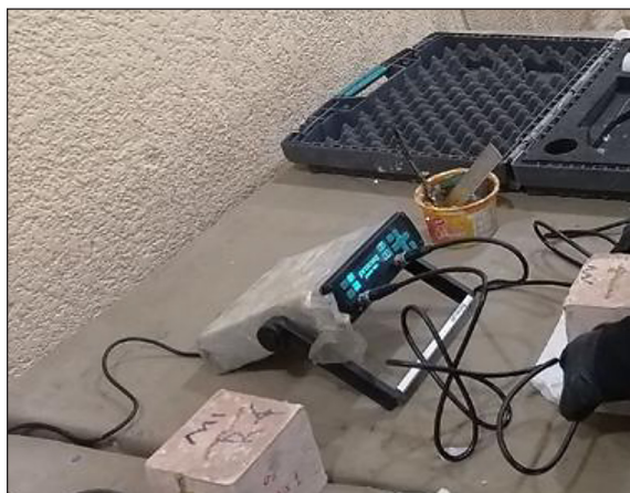
Figure 3. Ultrasonic pulse velocity test
