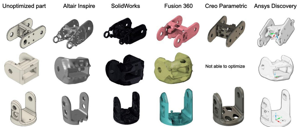
Figure 4. Three optimized arms after optimization. Five engineering software tools have been employed by the authors to optimize the arms based on specified criteria. The results propose that these platforms can effectively balance simplicity and complexity [55]
