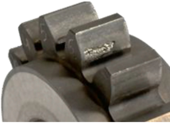
Figure 1. Pitting on the working surface of the gear tooth
