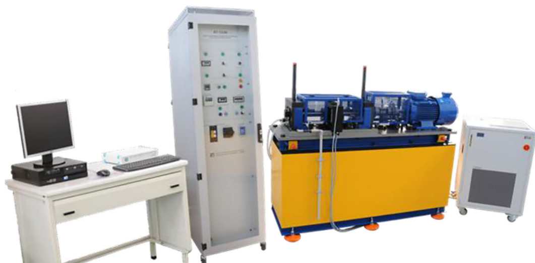
Figure 4. T-12U face-to-face gear test rig
