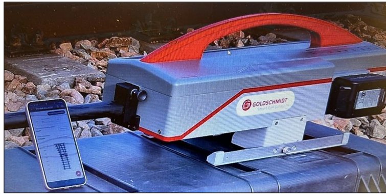
Figure 9. Laser profilometer „Railprofile 2D” SN005/23
