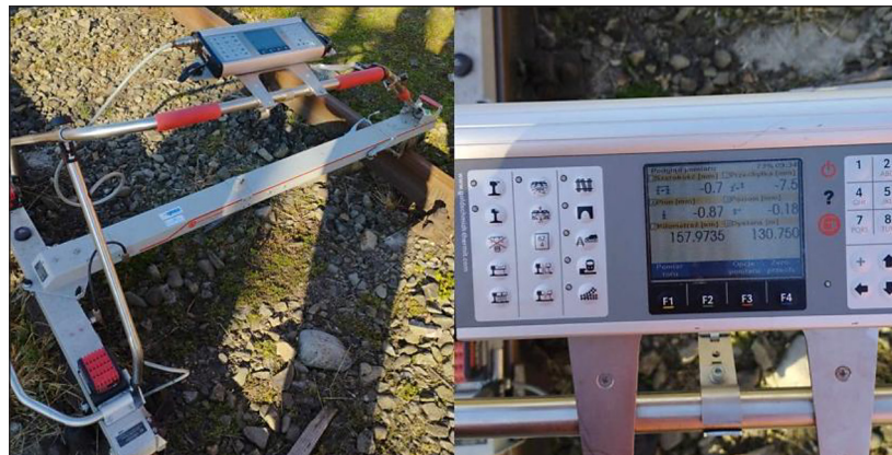
Figure 7. Digital track gauge
