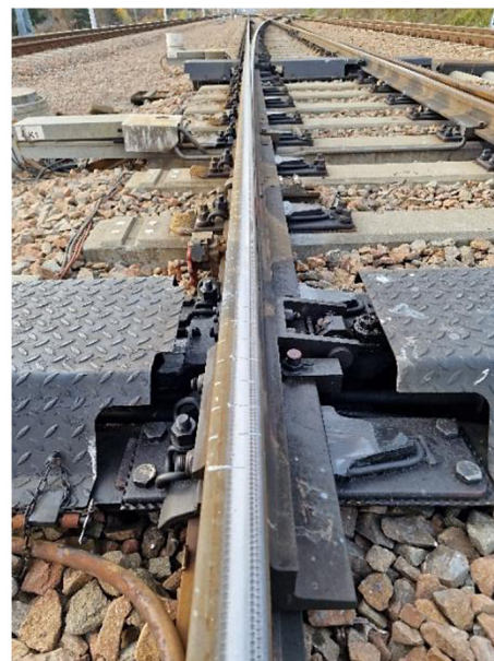
Figure 10. Tested switch: a) measurement of the curved switch rail, b) measurement locations
