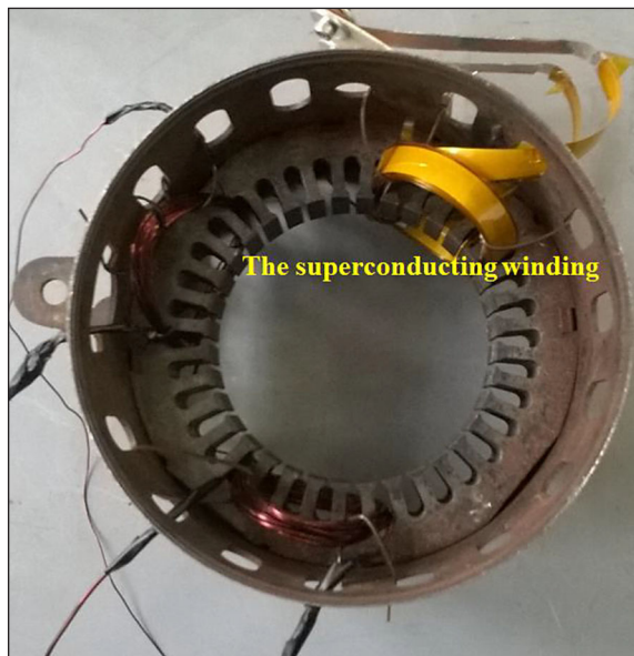
Figure 13. The superconducting winding mounted in slots of the stator of the generator
