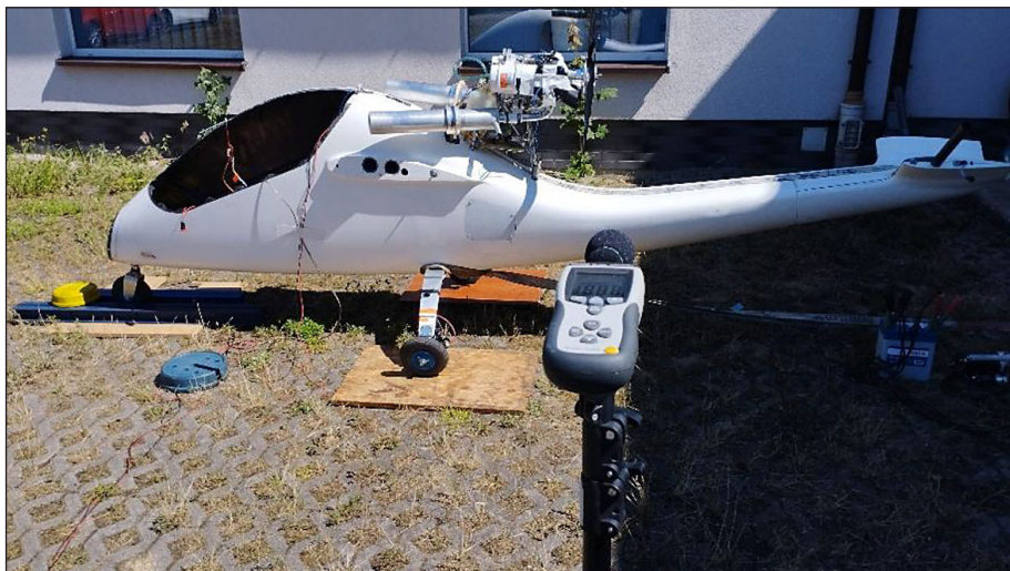
Figure 2. View of the load cell installation and the layout of test subsystems during thrust testing and noise-level measurement
