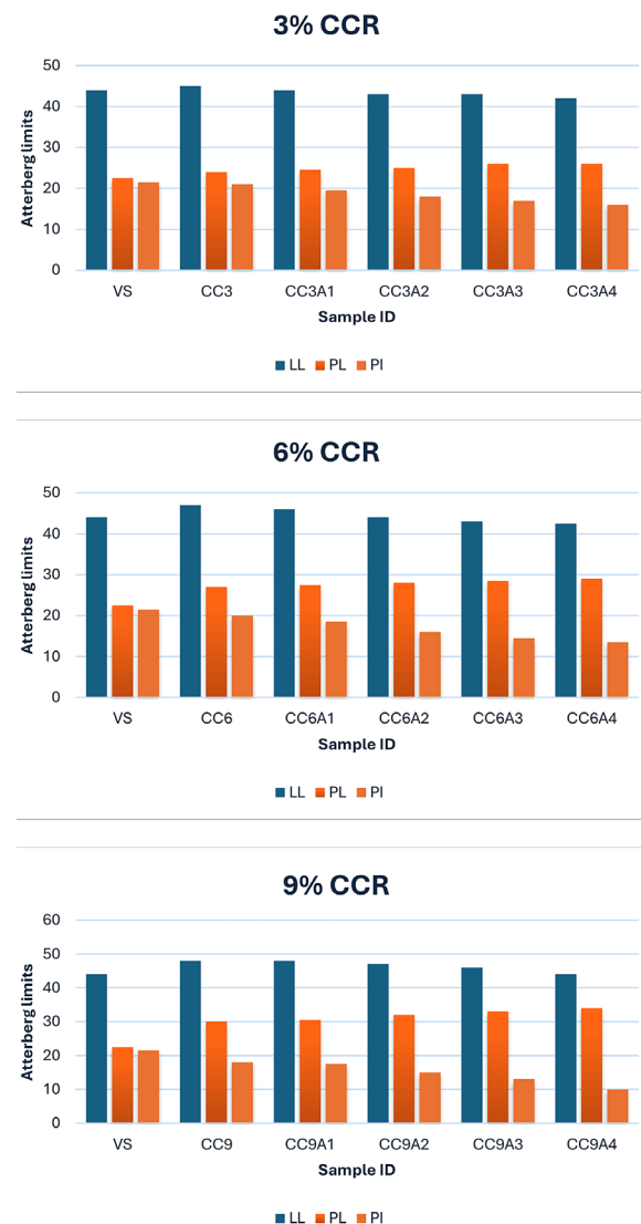
Figure 3. Atterberg limits tests results for calcium carbide residue ratios: (a) 3%, (b) 6%, (c) 9%
