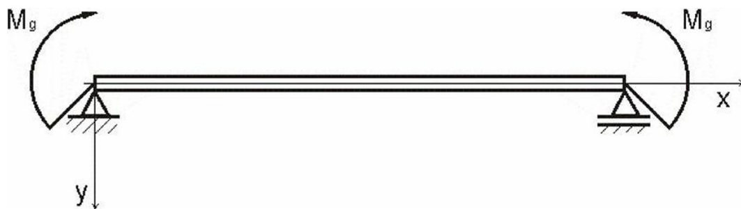
Figure 8. Clean bending: scheme
