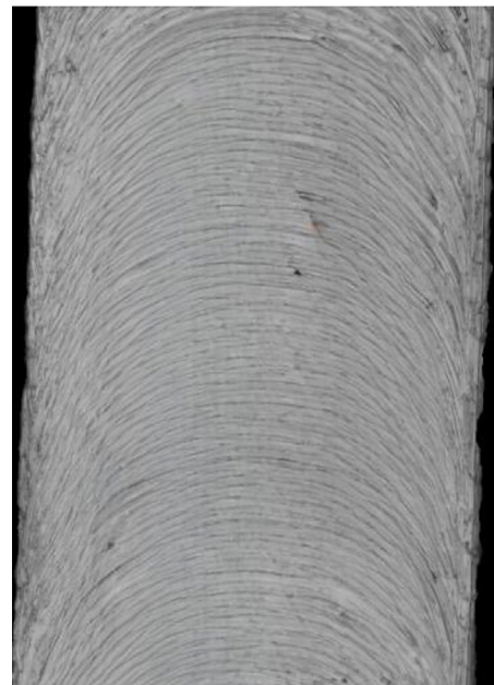
Figure 20. Surface with lowest roughness of 0.0384 microns
