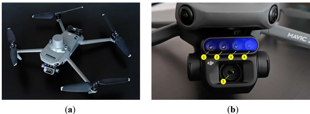
Figure 1. (a) Drone used for research and (b) multispectral camera on a drone: 1 – near-infrared lens; 2 – red edge band lens; 3 – red band lens; 4 – green band lens; 5 – RGB lens
