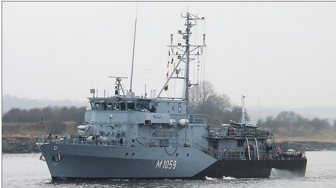
Figure 1. German Frankenthal class mine destroyer made of austenitic steel [16]
