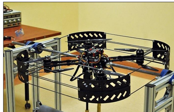
Figure 11. Testbed for UAV control system prototyping
