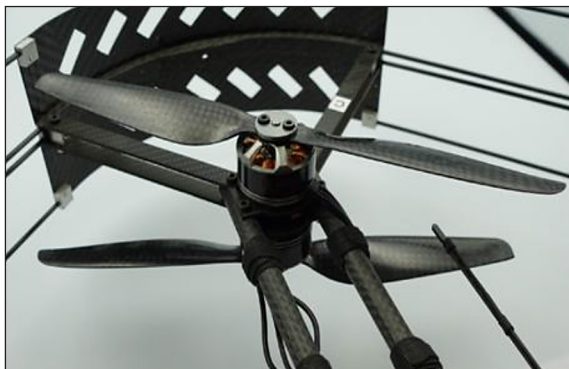
Figure 10. View on dual propeller system of Falcon V5
