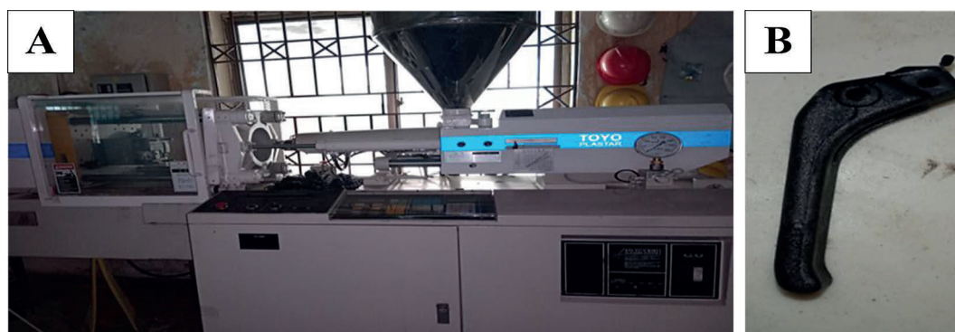
Figure 6. (A) Injection molding setup, (B) Injected part
