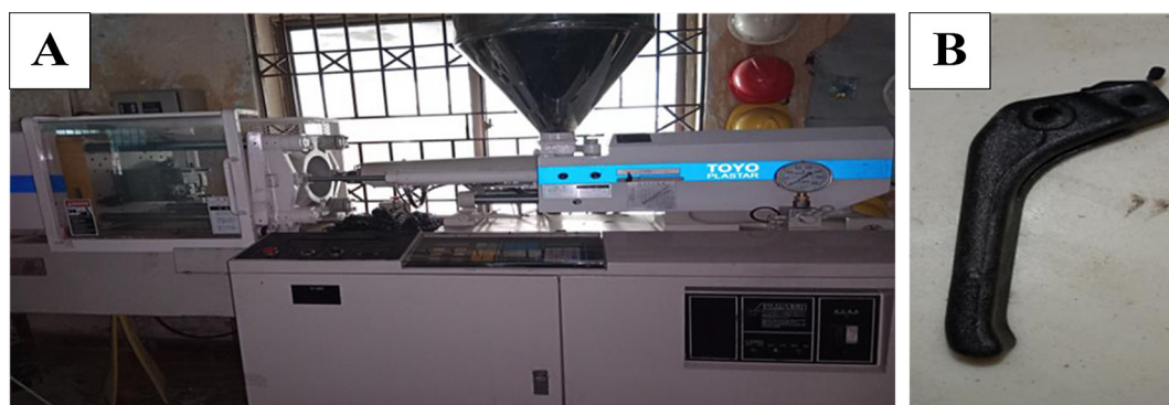
Figure 6. (A) Injection molding setup, (B) Injected part
