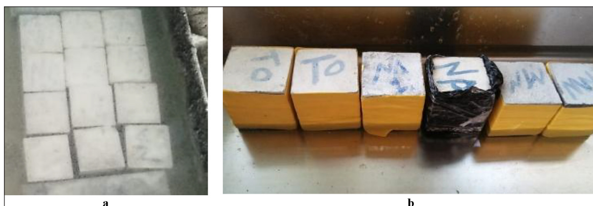
Figure 2. (a) Water absorption; (b) sorptivity
