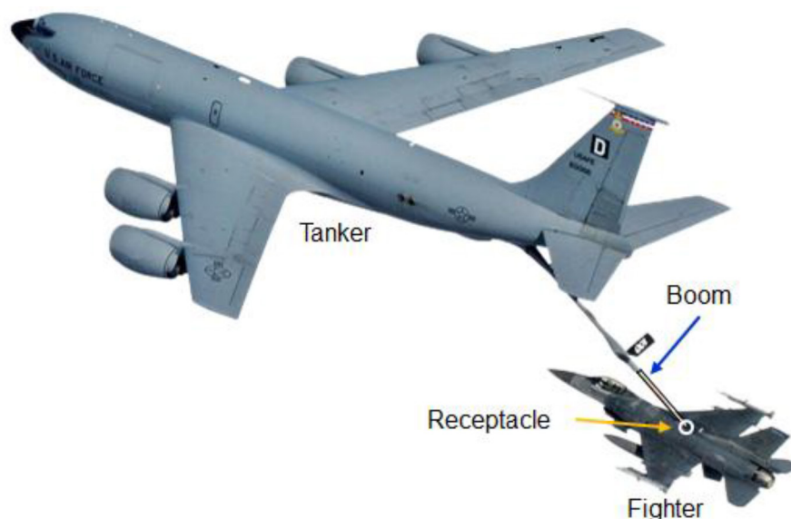
Figure 2. Flying boom system (boom and receptacle system)
