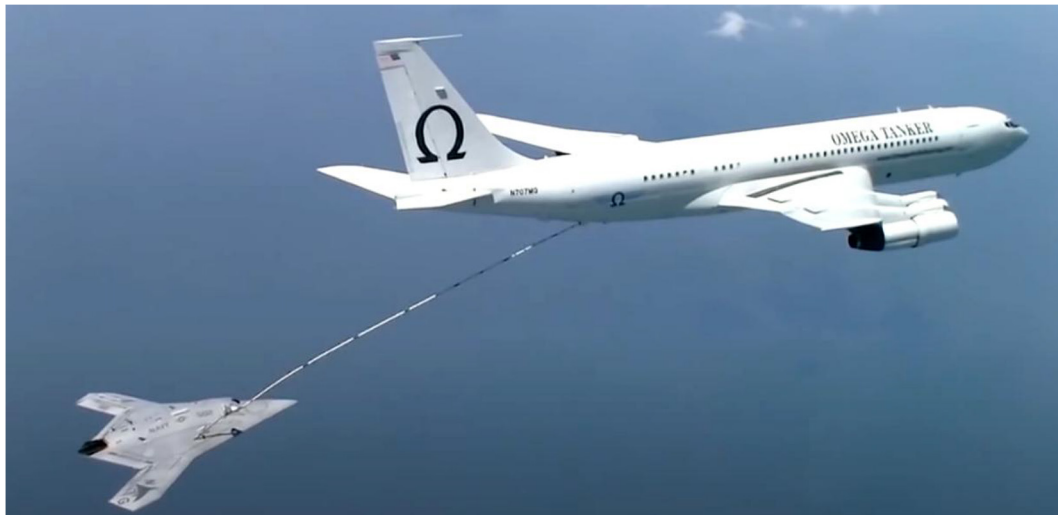
Figure 19. AAR system configuration with a probe and drogue model
