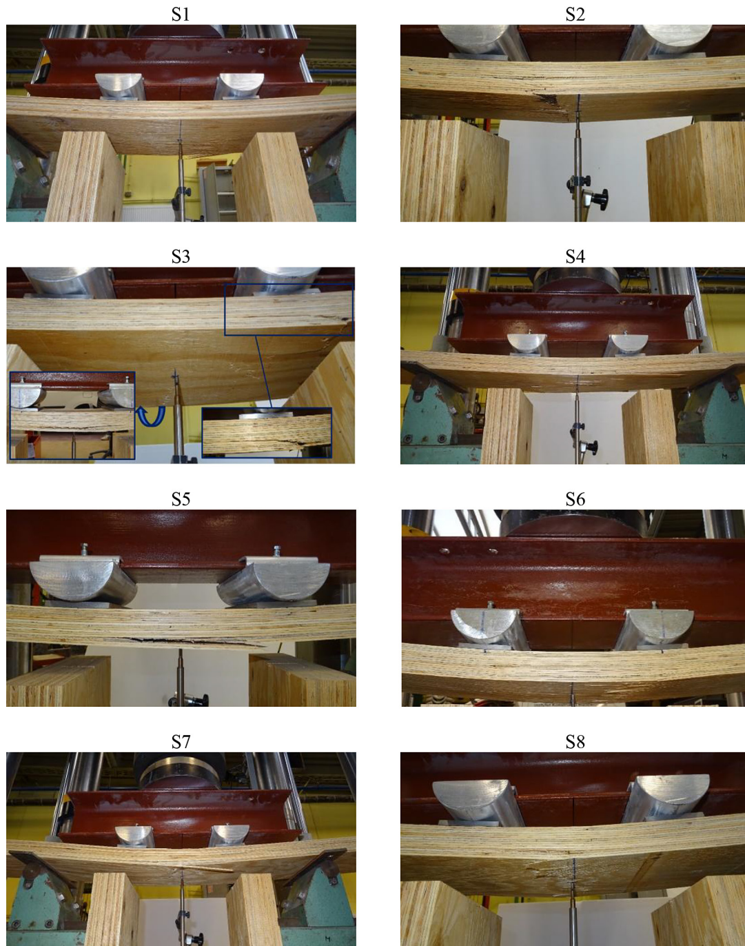
Figure 8. Failure modes of the LVL slabs
