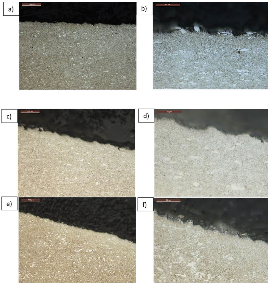
Figure 20. Microstructure of NC11LV steel in the near-surface region of the friction edge – light microscopy, etched state: a),b) 1020/200, c),d) 960/450, e),f) 1060/450
