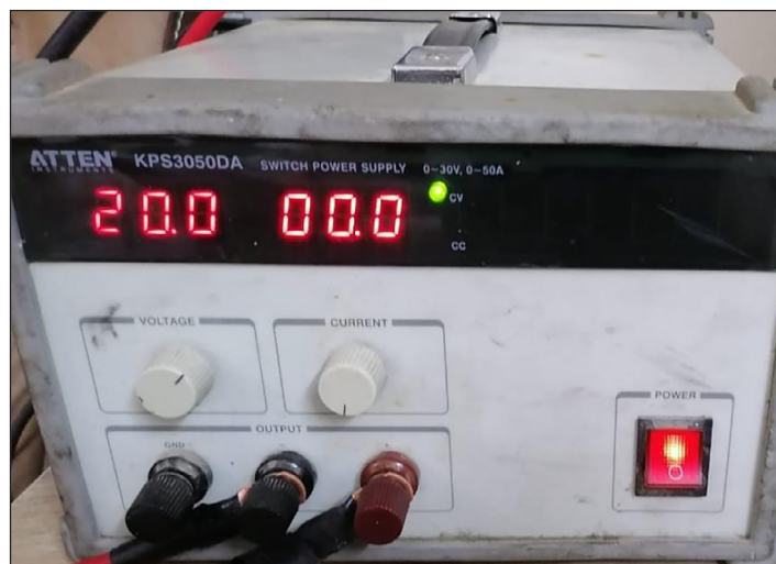
Figure 4. The power supply utilized in the experiments
