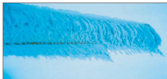
Figure 2. Accumulation of ice layers on wind turbine blades (51)
