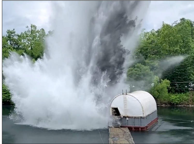
Fig. 1. Typical MIL-DTL-901E floating shock platform setup [19, 20]
