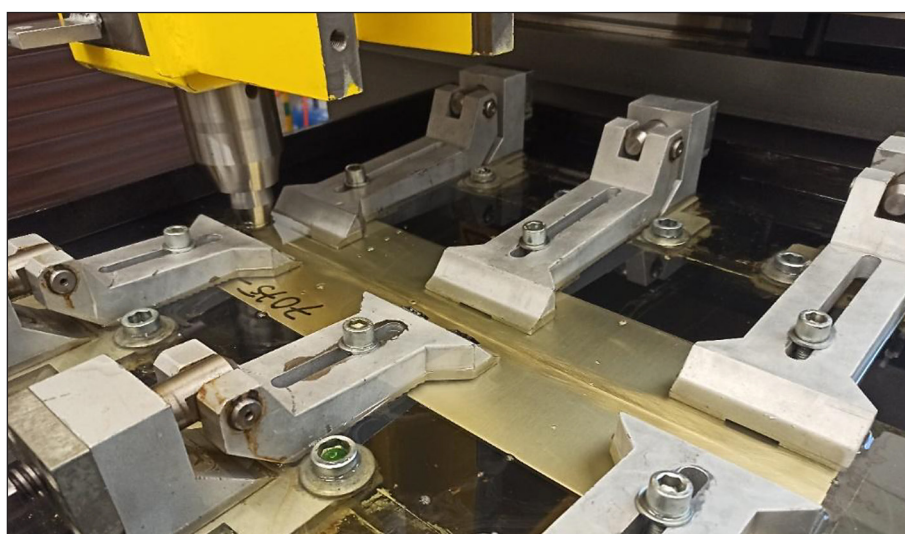
Figure 1. The welding setup shown using quenching oil as the cooling medium
