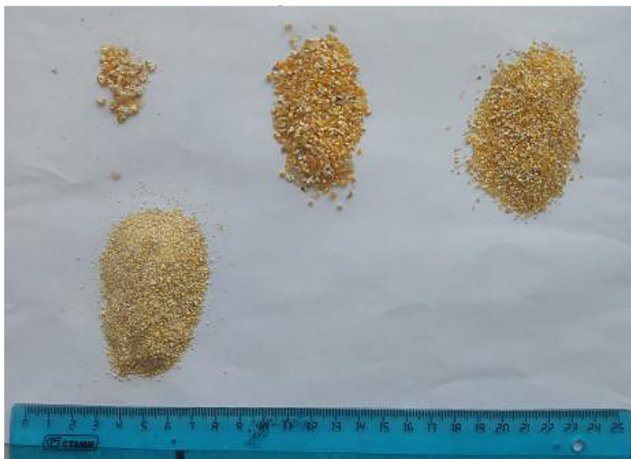
Figure 5. Photo of the results of the sieve analysis of the crushed grain corn
