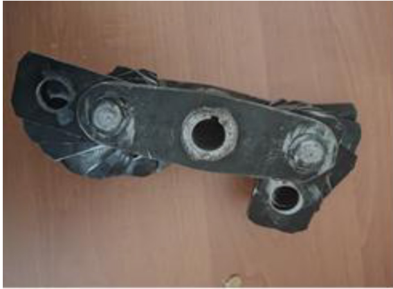
Figure 3. Rotor with two sets of hammers with angles of inclination of 60^\circ on both ends
