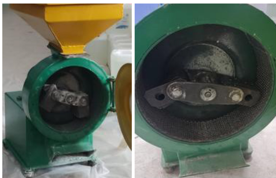
Figure 2. Hammer crusher DIK-1.5: a – overall view; b – grinding chamber
