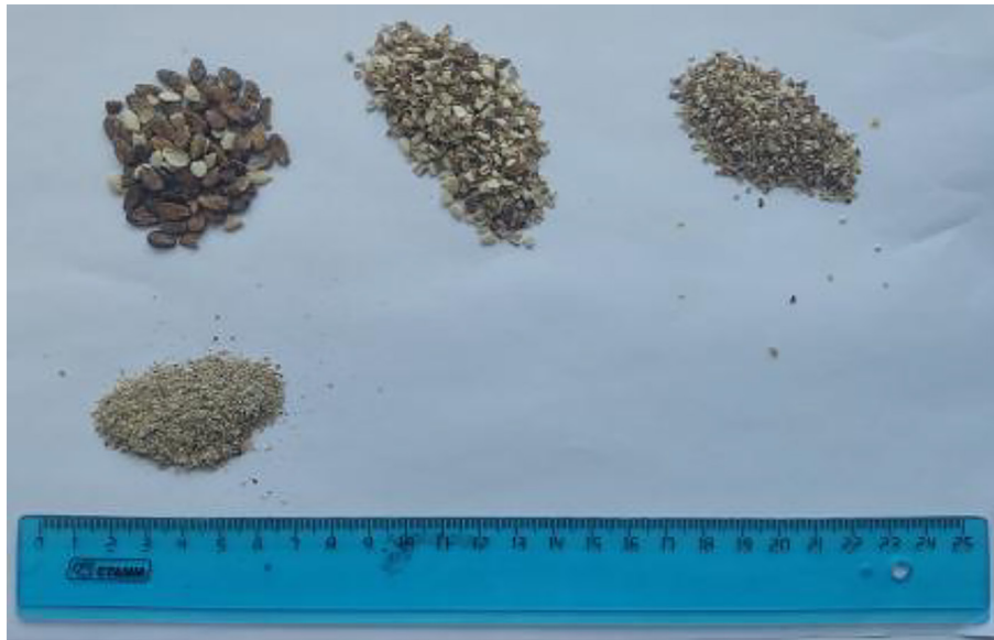
Figure 7. Photo of the results of the sieve analysis of ground watermelon seeds
