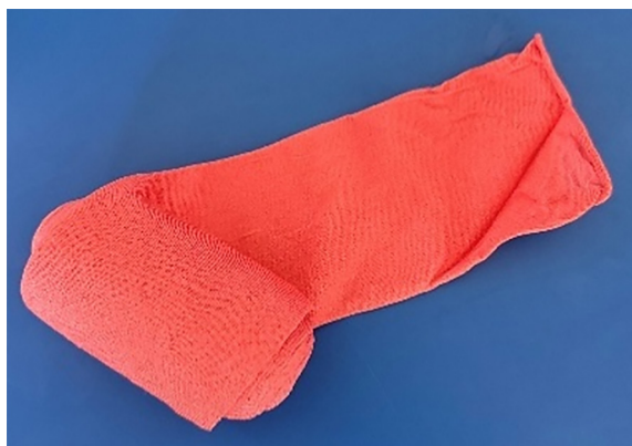
Figure 5. PL-3 polypropylene fibre knitted fabric
