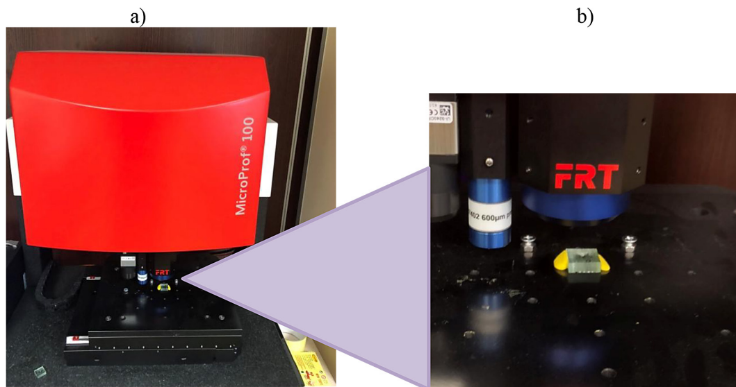
Figure 8. MicroProf 100 device: a) general view, b) specimen mouting method
