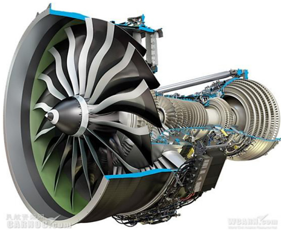
Figure 6. GE9X engine cross section visualization [24]
