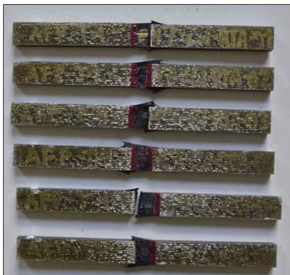
Figure 12. Compression 0° samples with tabs
