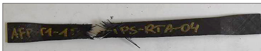
Figure 10. Break at 40 mm elongation and 8 mm necking
