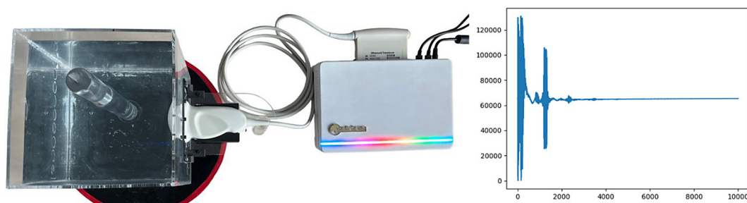
Figure 5. The third version of the tomograph is used to study the lower urinary tract during measurements on phantoms, along with the measured signal from a single channel of the ultra-sound transducer head
