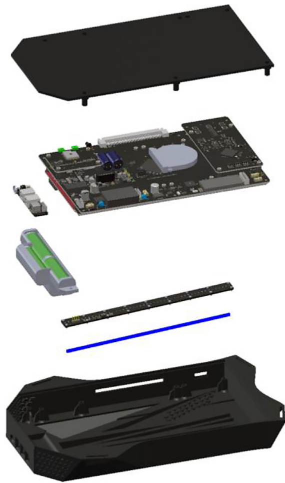
Figure 6. 3D model of UST & EIT tomograph construction
