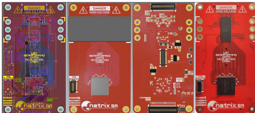
Figure 11. Ultrasound 8-channel beamforming measuring card
