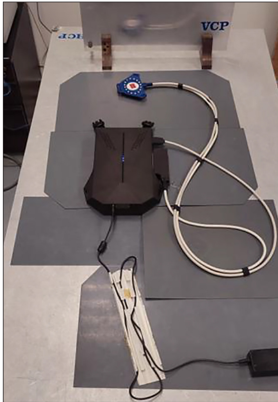
Figure 20. UST/EIT tomograph during ESD immunity tests
