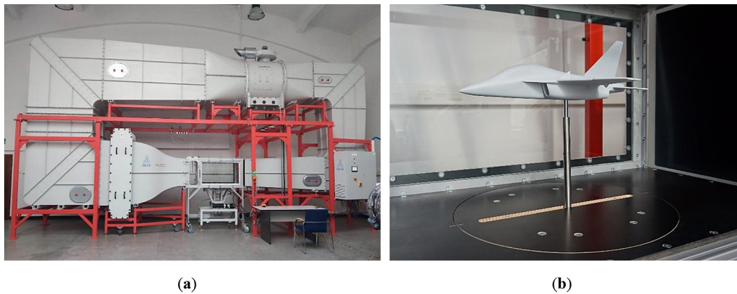
Figure 1. (a) Wind tunnel used for experimental studies and (b) a view of the test object (an Alenia Aermacchi M-346 Master model) during wind tunnel testing [43]
