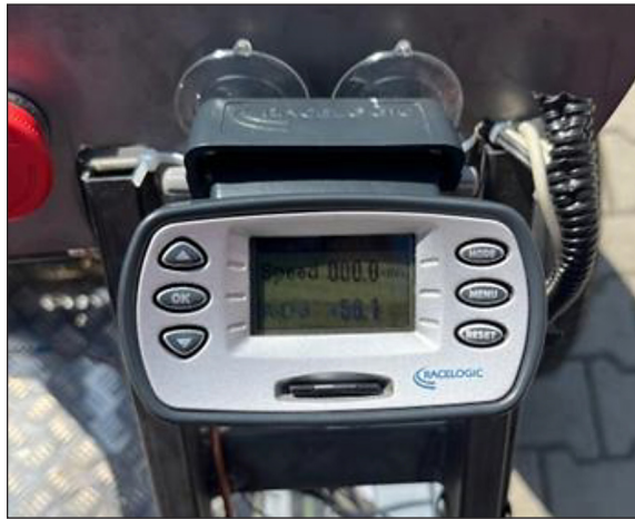
Figure 5. Racelogic PerformanceBox device mounted on the vehicle during testing
