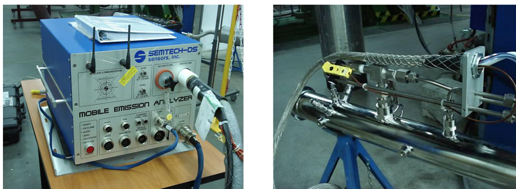
Figure 5. SEMTECH DS analyzer and flow meter for measuring exhaust gas mass flow rate
