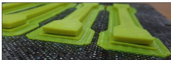
Figure 3. Samples made of PC/ABS material with full density internal structure on the UP BOX+ printer
