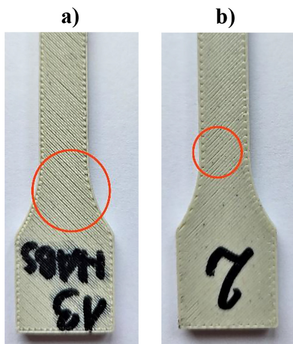
Figure 9. H13 samples in bottom view (a) and top view (b) with marked underfills
