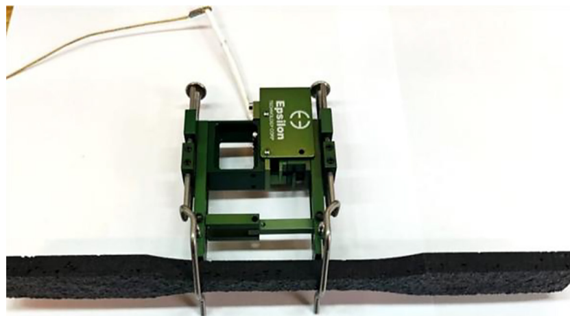
Figure 11. Epsilon 3542 strain gauge installed on a specimen prepared for a static tensile test
