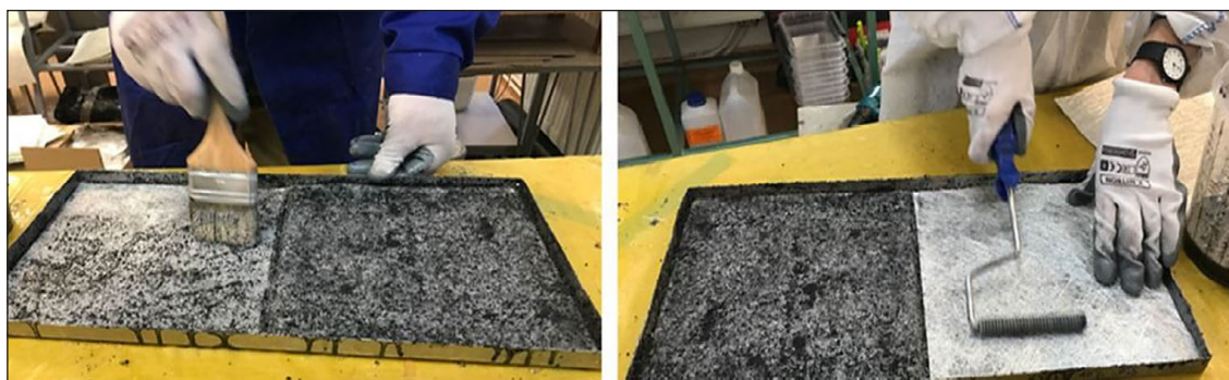
Figure 8. Method of hand lamination of the composite to be tested
