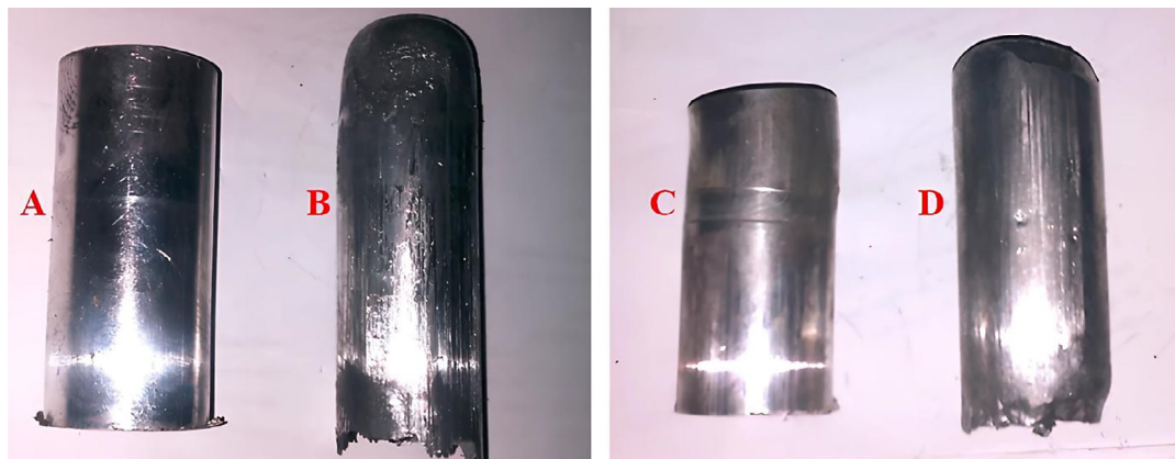
Figure 7. Photograph of EN AW-1050A aluminum after first extrusion (A – first sample; B – second sample extruded immediately after the first) and second extrusions (C – sample prepared for the next operation; D – sample after removal from the punch)
