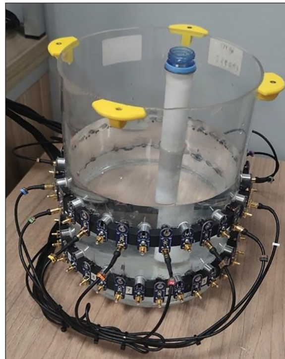
Figure 2. Test tank used for calibration and verification of the EIT device. Inside the tank there is a phantom made of plastic that imitates the conductive properties of biological tissues. On the inner surface of the tank wall, 16 measuring electrodes are placed evenly distributed in one plane. The electrodes are used to cyclically measure voltage and current as part of the measurement sequence. This arrangement allows for simulation of the conditions of a real examination of the urinary bladder using an impedance tomography system
