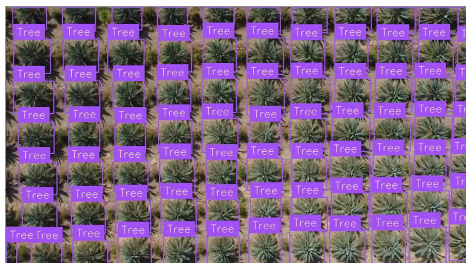
Figure 9. The example of the result of palm crowns detection from altitude 100 meters
