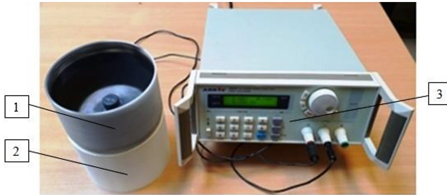
Figure 2. View of the test stand used to test the density distribution of rotating fluids: 1 – rotating vessel, 2 – low-speed electric motor, 3 – electric power supply
