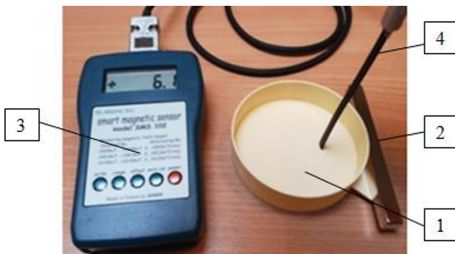
Figure 8. Test stand for testing the density distribution after magnet application: 1 – vessel equipped with a magnet holder, 2 – neodymium bar magnet, 3 – induction meter, 4 – measuring probe
