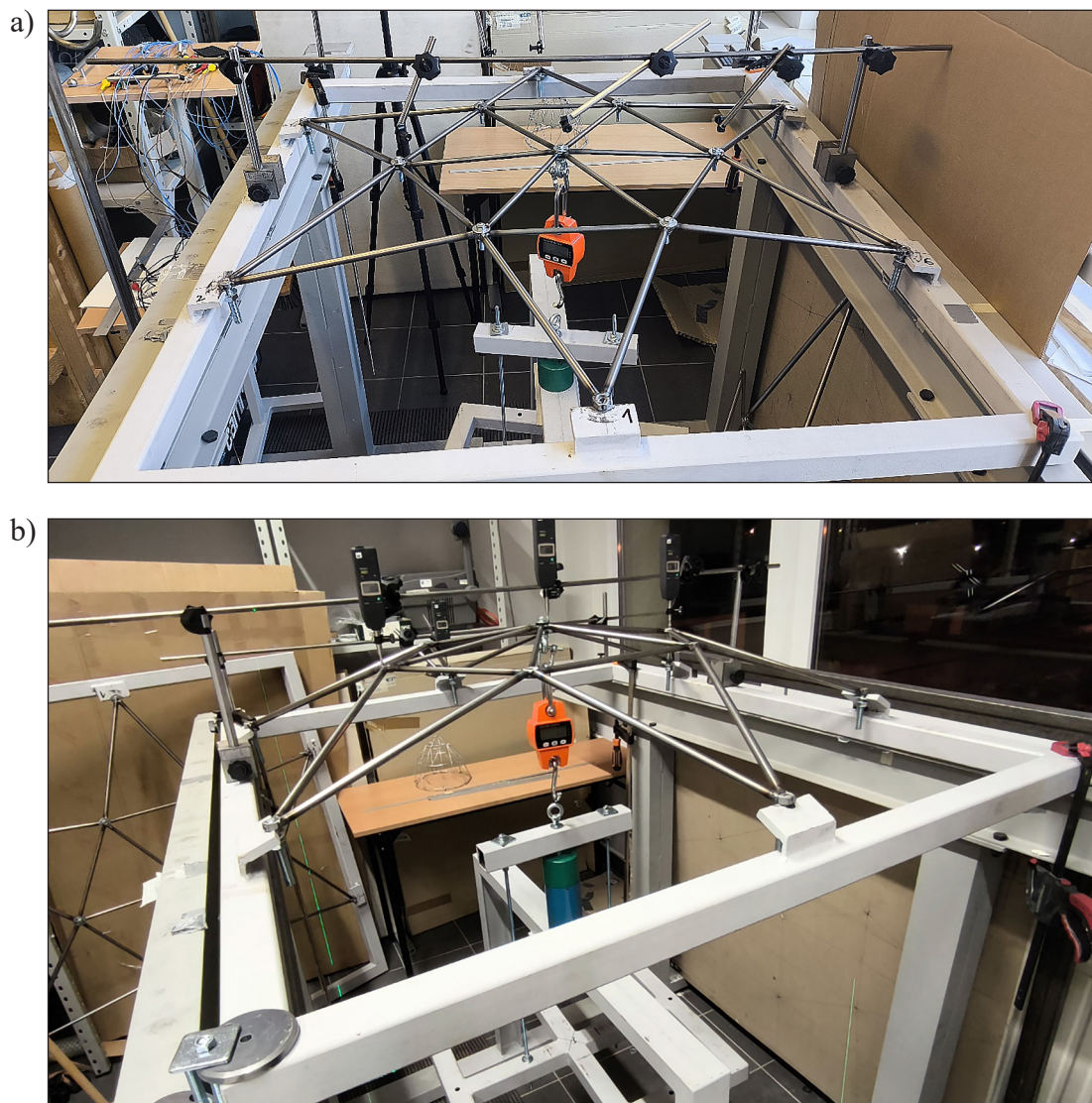
Figure 4. Experimental model: (a) low-rise dome, (b) high-rise dome
