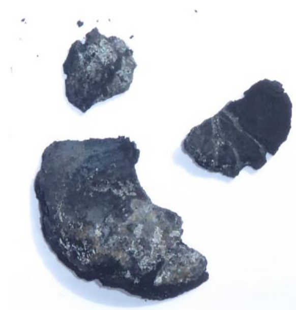
Figure 12. Slag deposit obtained from the nozzle converging section
