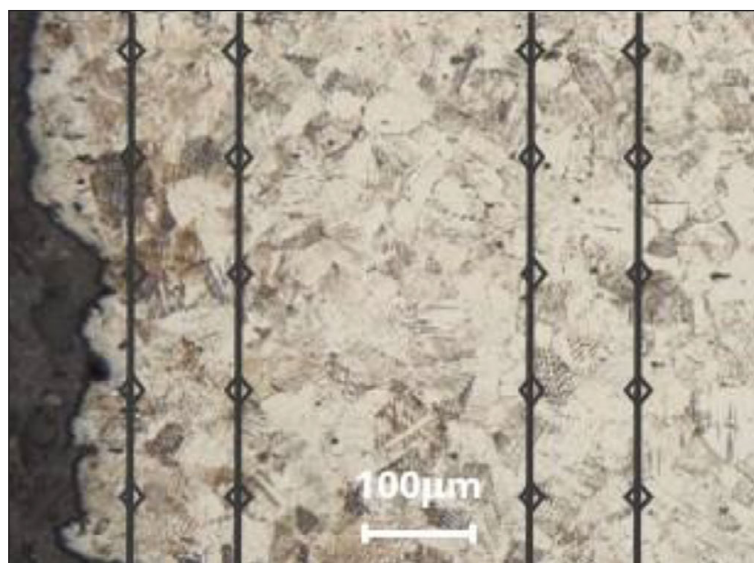
Figure 6. Schematic showing hardness measurement locations on the deposit after fatigue testing
