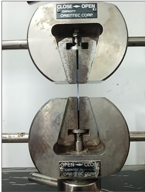
Figure 7. Specimen on the tensile testing machine
