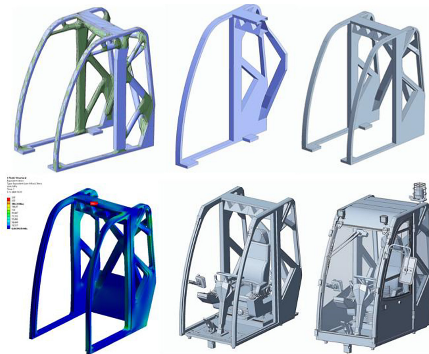
Figure 4. Modification of area modelling and final TO cab assembly
