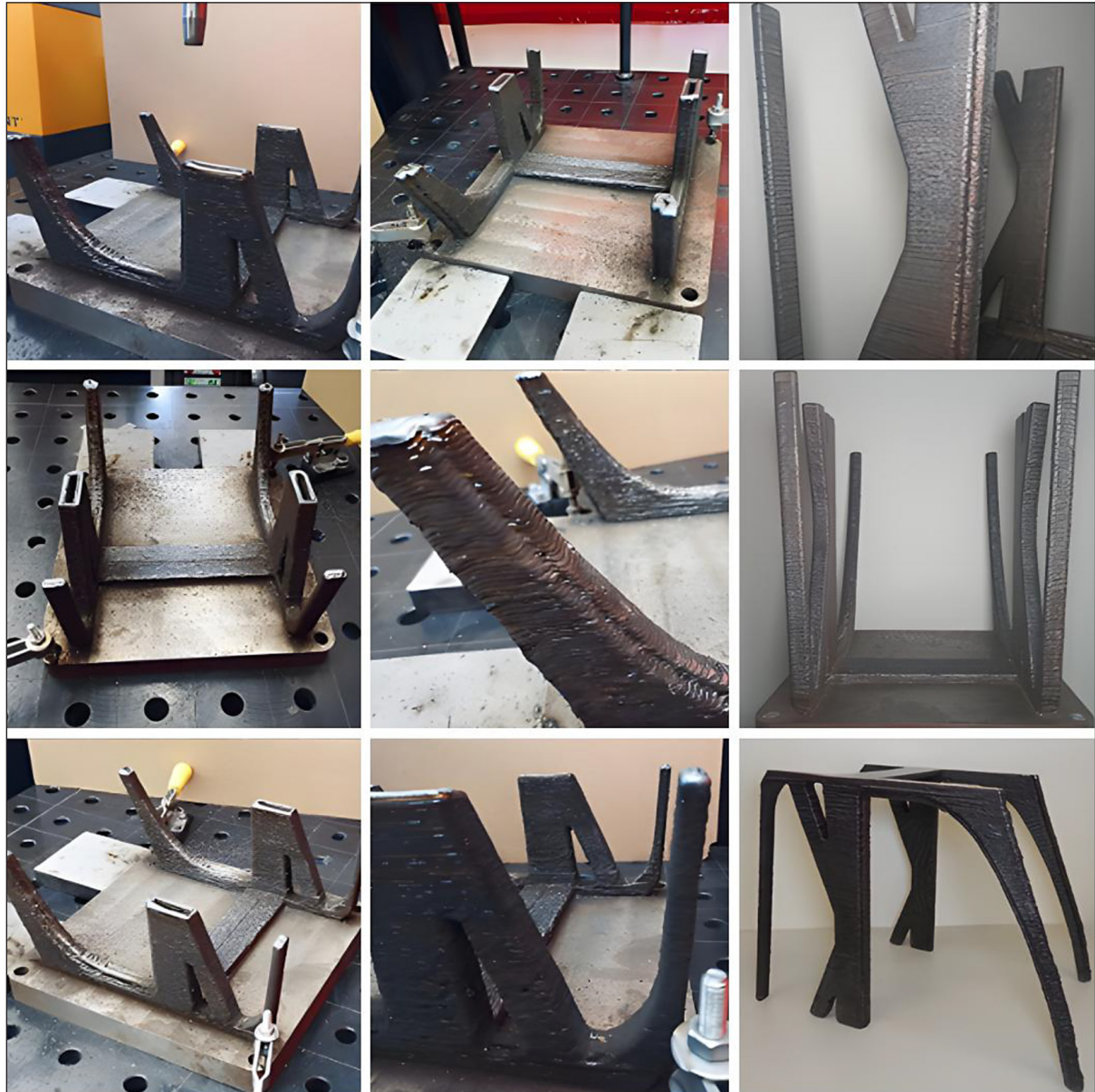
Figure 7. Part of the frame module made by WAAM technology
