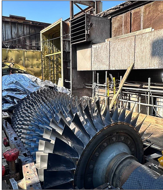
Figure 3. Compressor blades of frame 9 from GE company
