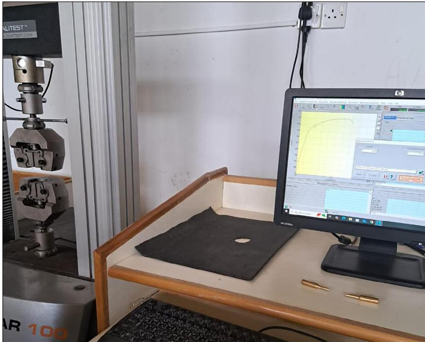
Figure 5. The Instron tensile machine with the fractured tool
