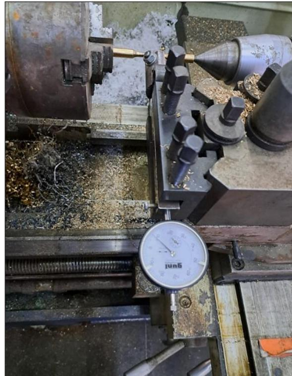
**Figure 1.** Burnishing tool and lath machine
