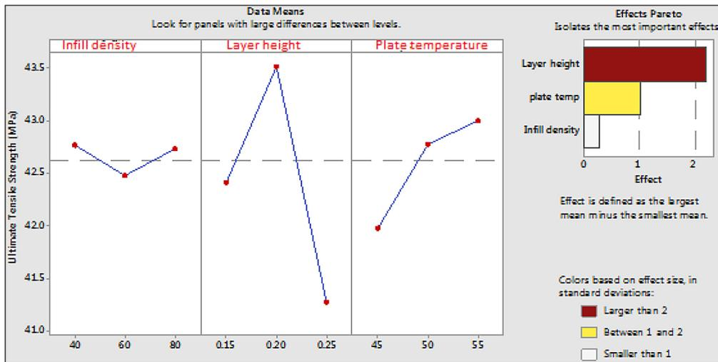
Figure 6. The main effects screener for tensile strength
