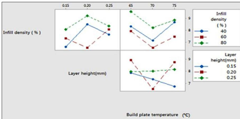
Figure 9. Surface roughness interaction plot
