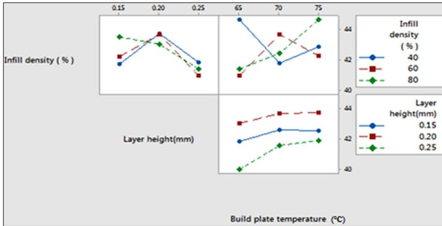
Figure 8. Tensile strength's interaction plot
