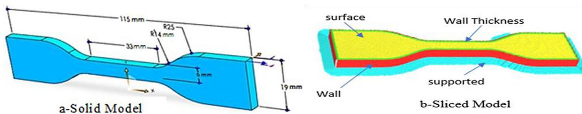
Figure 2. Solid and sliced models for tensile specimens
