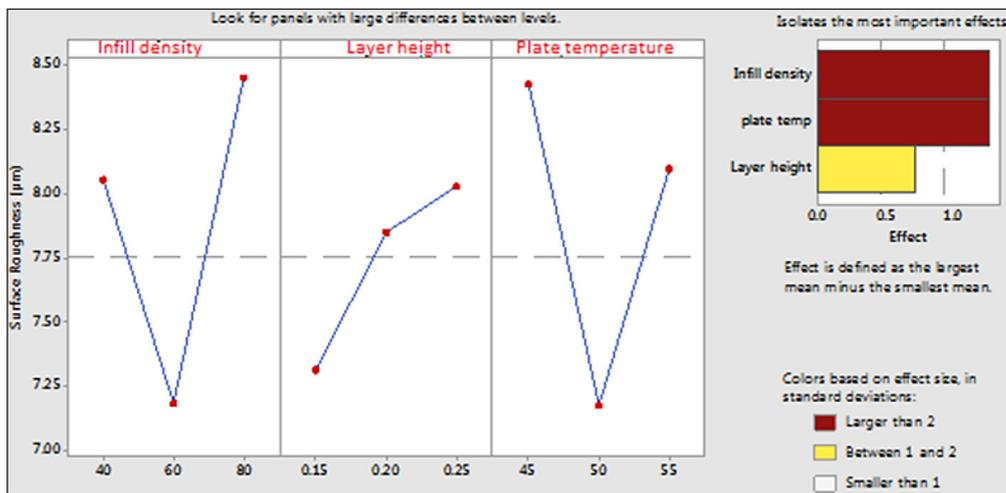
Figure 7. The main effect screener for surface roughness
