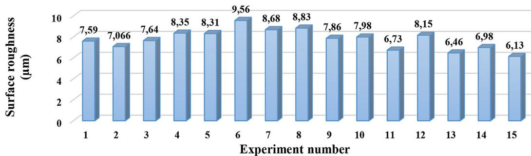
Figure 5. Surface roughness of PETG printed specimens
