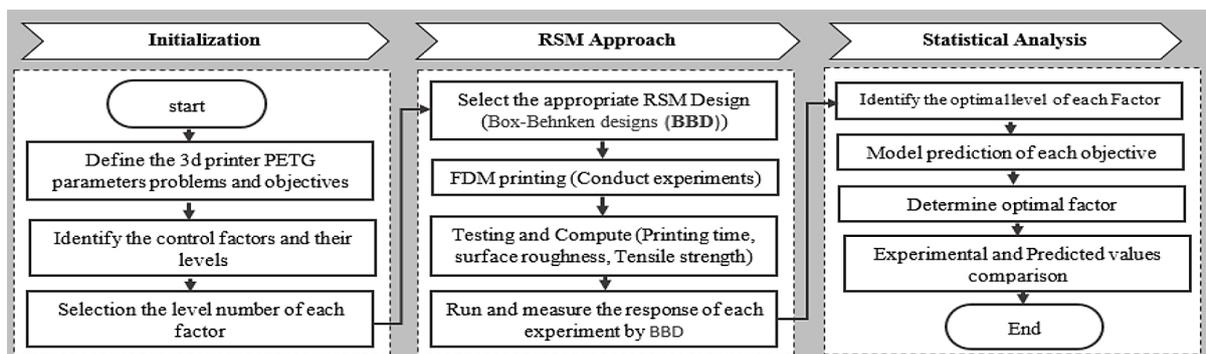
**Figure 3.** Overview of process parameters optimization and prediction methodology
