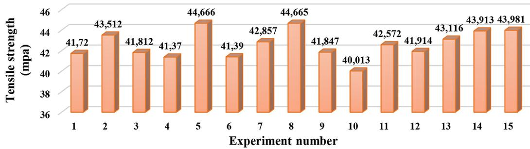
Figure 4. Tensile strength of PETG printed specimens
