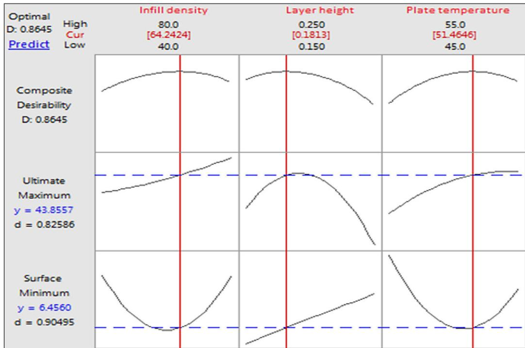
Figure 12. Optimization of tensile strength and surface roughness
