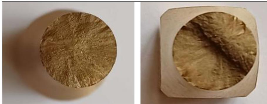
Figure 1. Classic fatigue crack surfaces after tensile-compressive and pendulum bending tests and RG7 bronze with a diameter of 10 mm at the narrowing point
