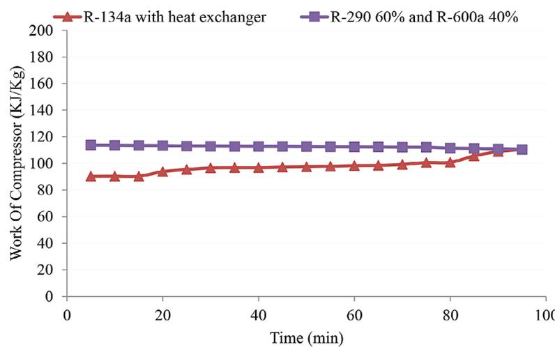
Figure 8. R134a work of compressor compare with (60%/40%) R290/R600a
