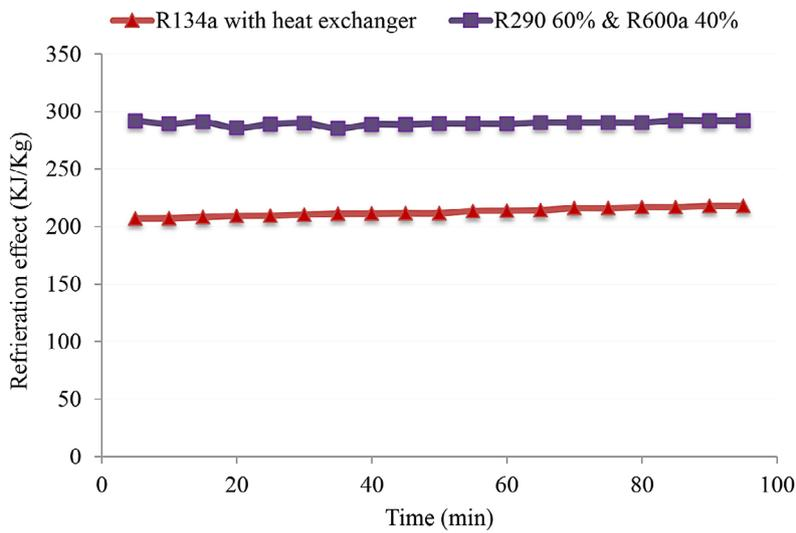
Figure 7. R134a refrigerating effect compare with (60 %/40%) R290/R600a
