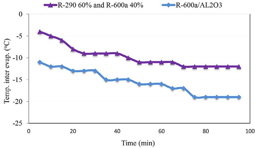
Figure 12. Comparison temp. inter evap. between (60 %/40 %) R290/R600a & R600a/Al<sub>2</sub>O<sub>3</sub>
