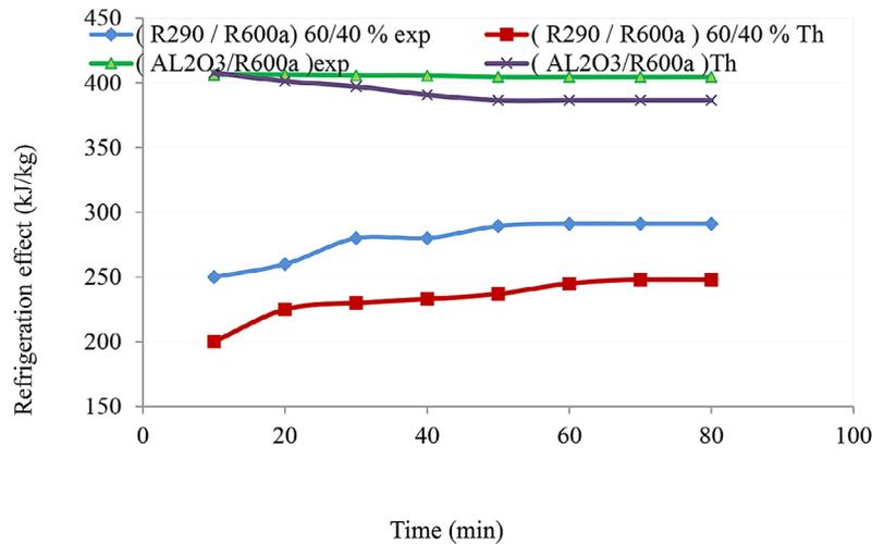
Figure 16. Difference between experimental & theoretical result of refrigerating effect for (60 /40)% R290/R600a & R600a/Al<sub>2</sub>O<sub>3</sub>
