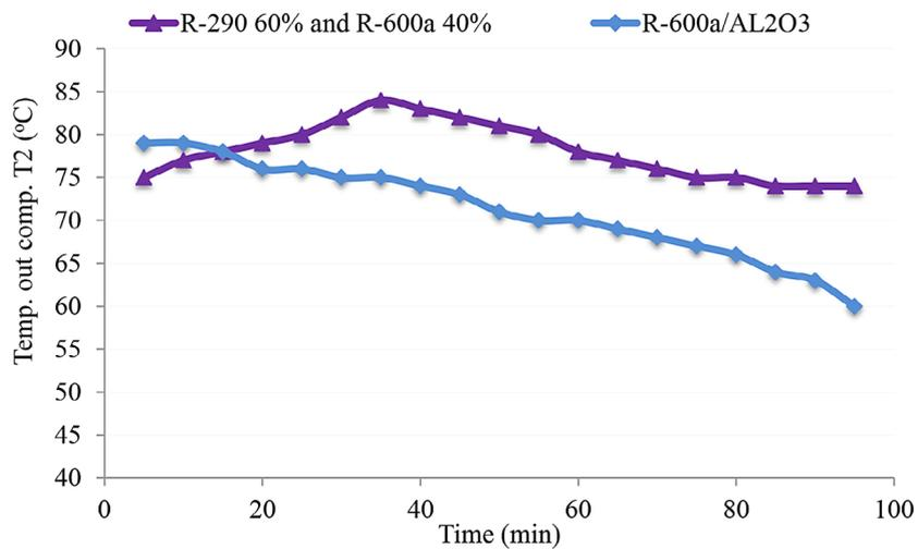
Figure 13. Comparison temp. out comp. T2 between (60 %/40 %) R290/R600a & R600a/Al<sub>2</sub>O<sub>3</sub>
