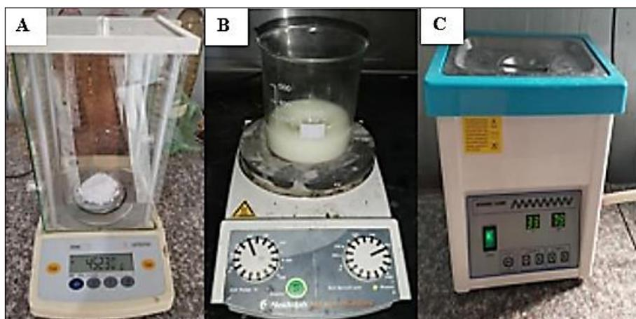
**Figure 4.** Equipment used in the preparation of nano-fluid: (A) electronic balance, (B) stirring hotplate, (C) ultrasonic device (16)
