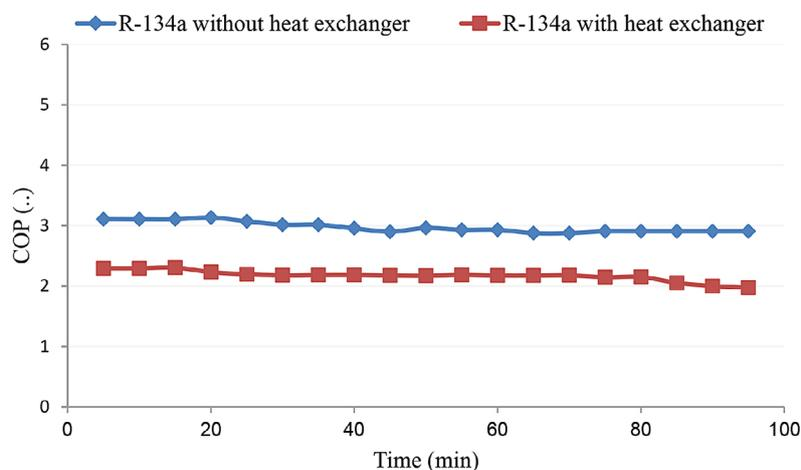
Figure 5. COP of the system in base operation with R134a
