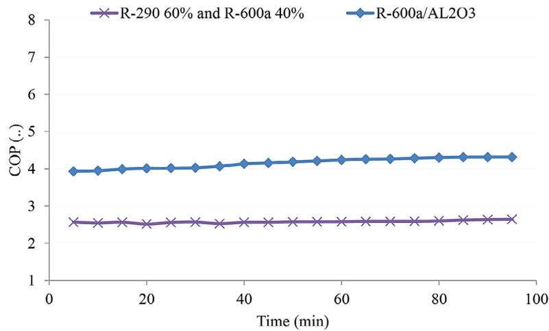
**Figure 9.** Comparison COP between (60%/40%) R290/R600a & R600a/Al<sub>2</sub>O<sub>3</sub>
