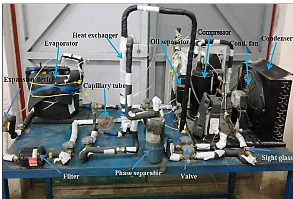
Figure 3. Experimental setup of vapour compression system
