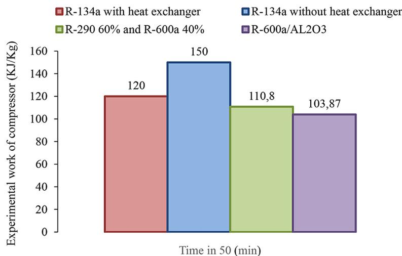
Figure 17. Experimental work of compressor in ambient temperature 48 °C for all refrigerants
