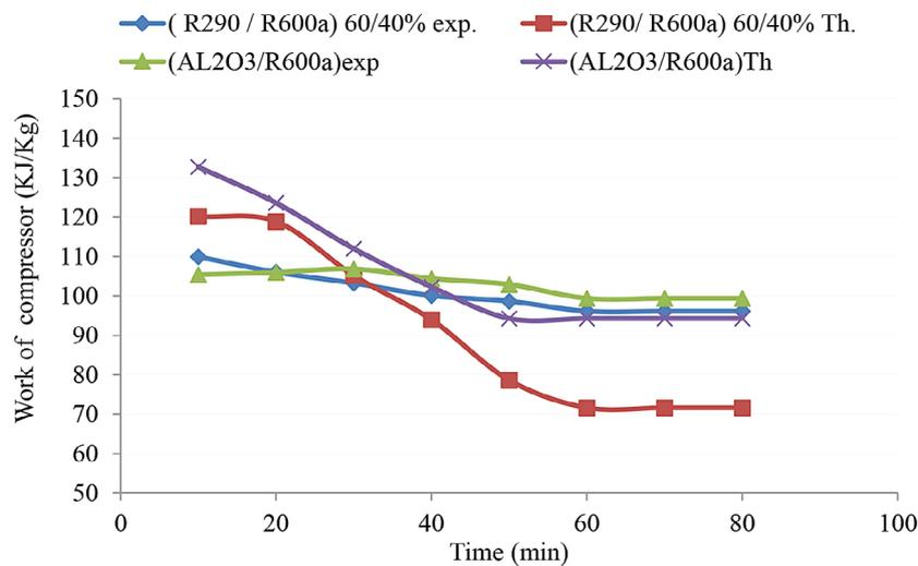
Figure 15. Difference between experimental & theoretical result of work of compressor for (60 /40)% R290/R600a & R600a/Al<sub>2</sub>O<sub>3</sub>
