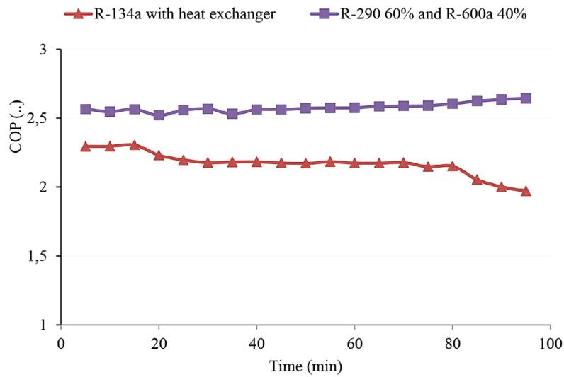
Figure 6. R134a with heat exchanger COP compare with (60%/40%) R290/R600a
