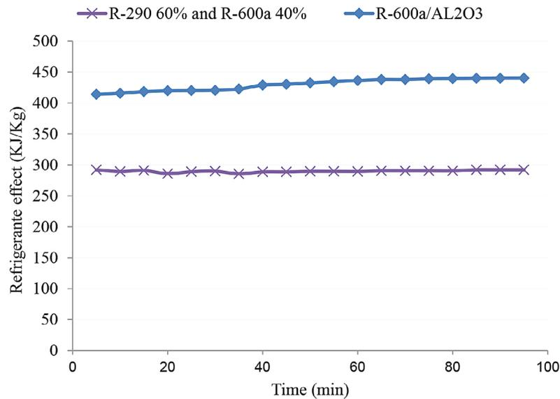
**Figure 10.** Comparison refrigerating effect between (60%/40%) R290/R600a & R600a/Al<sub>2</sub>O<sub>3</sub>
