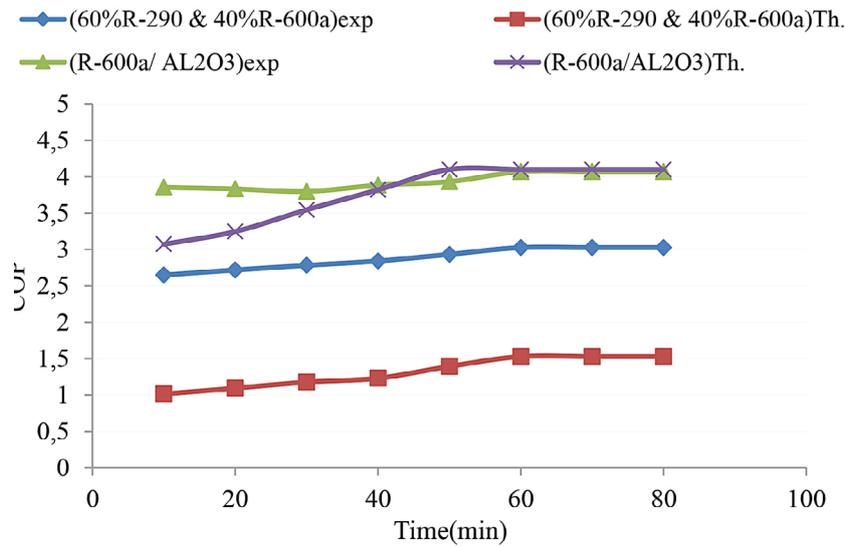
Figure 14. difference between experimental & theoretical result of COP for (60 /40) % R290/R600a & R600a/Al<sub>2</sub>O<sub>3</sub>
