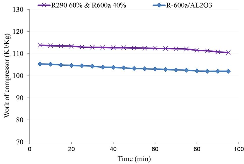
Figure 11. Comparison work of compressor between (60%/40%) R290/R600a & R600a/Al<sub>2</sub>O<sub>3</sub>
