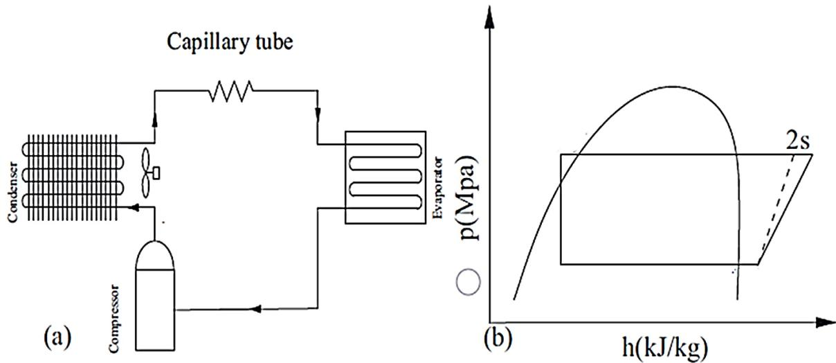
Figure 1. (a) schematic of vapour compression system, (b) p-h diagram of VCP (23)
