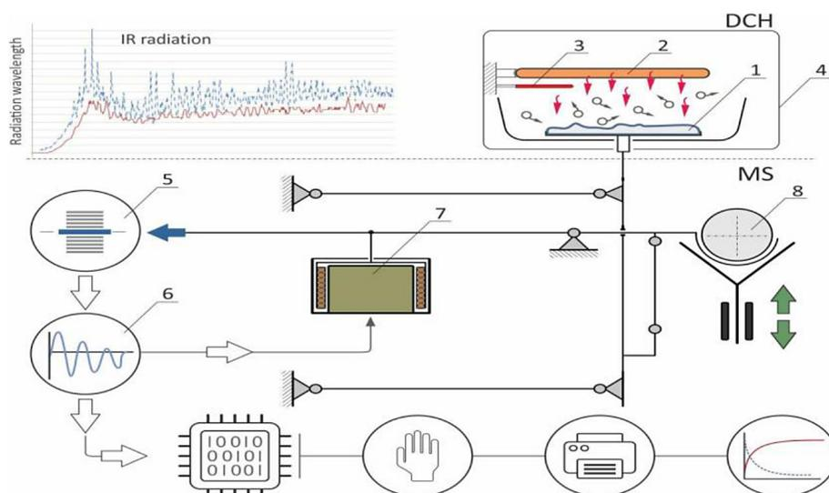
**Figure 3.** Diagram of the operating principle of the moisture analyzer
