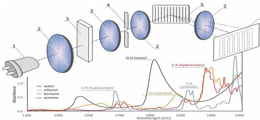
**Figure 2.** General diagram explaining on how NIR technology works. Legend: 1 – NIR LED, 2 – lens, 3 – sample, 4 – slit, 5 – greting, 6 – detector array (own work)
