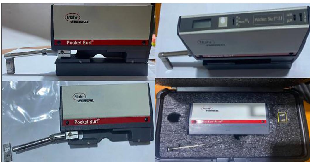
Figure 6. The Ra tester pocket surf device
