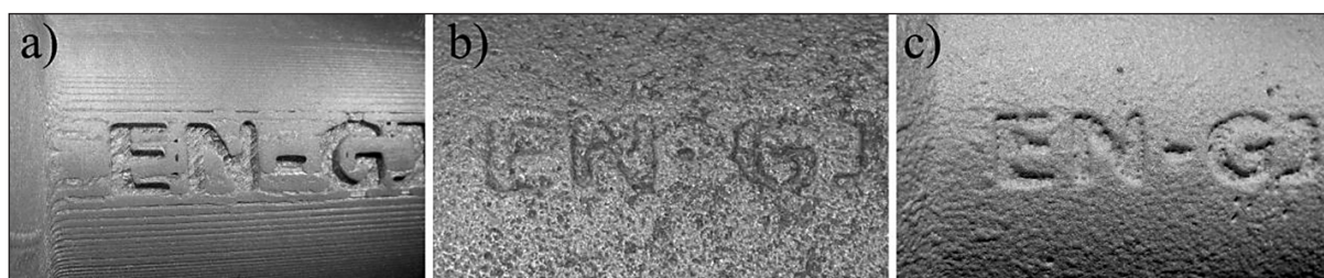
Figure 19. Reproducing letters at: (a) printed model, (b) cast iron casting, (c) aluminum-silicon casting
